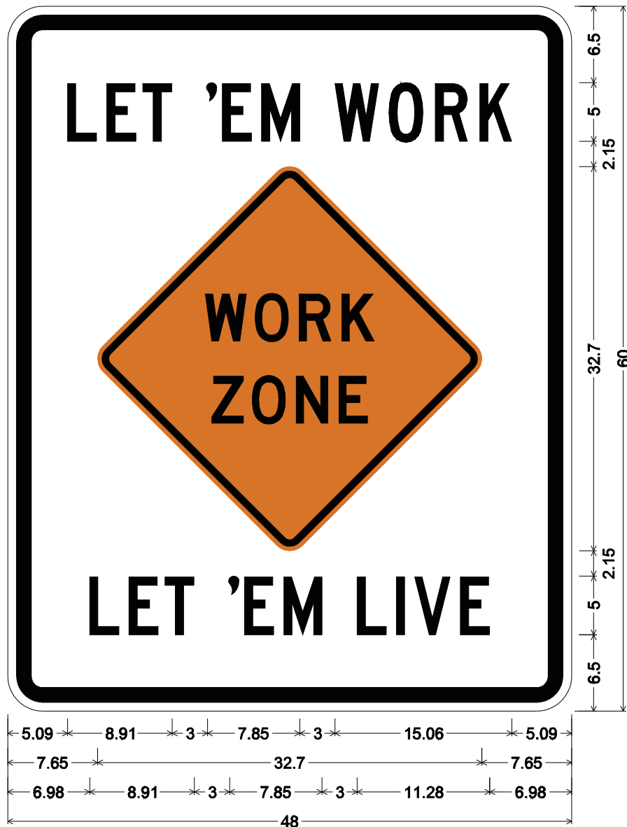
G20-5-48; 3.00" Radius, 1.25" Border, 0.75" Indent, Black on White; [LET] C; ['EM] C; [WORK] C; ssas; [LET] C; ['EM] C; [LIVE] C; Table of distances between letter and object lefts.
