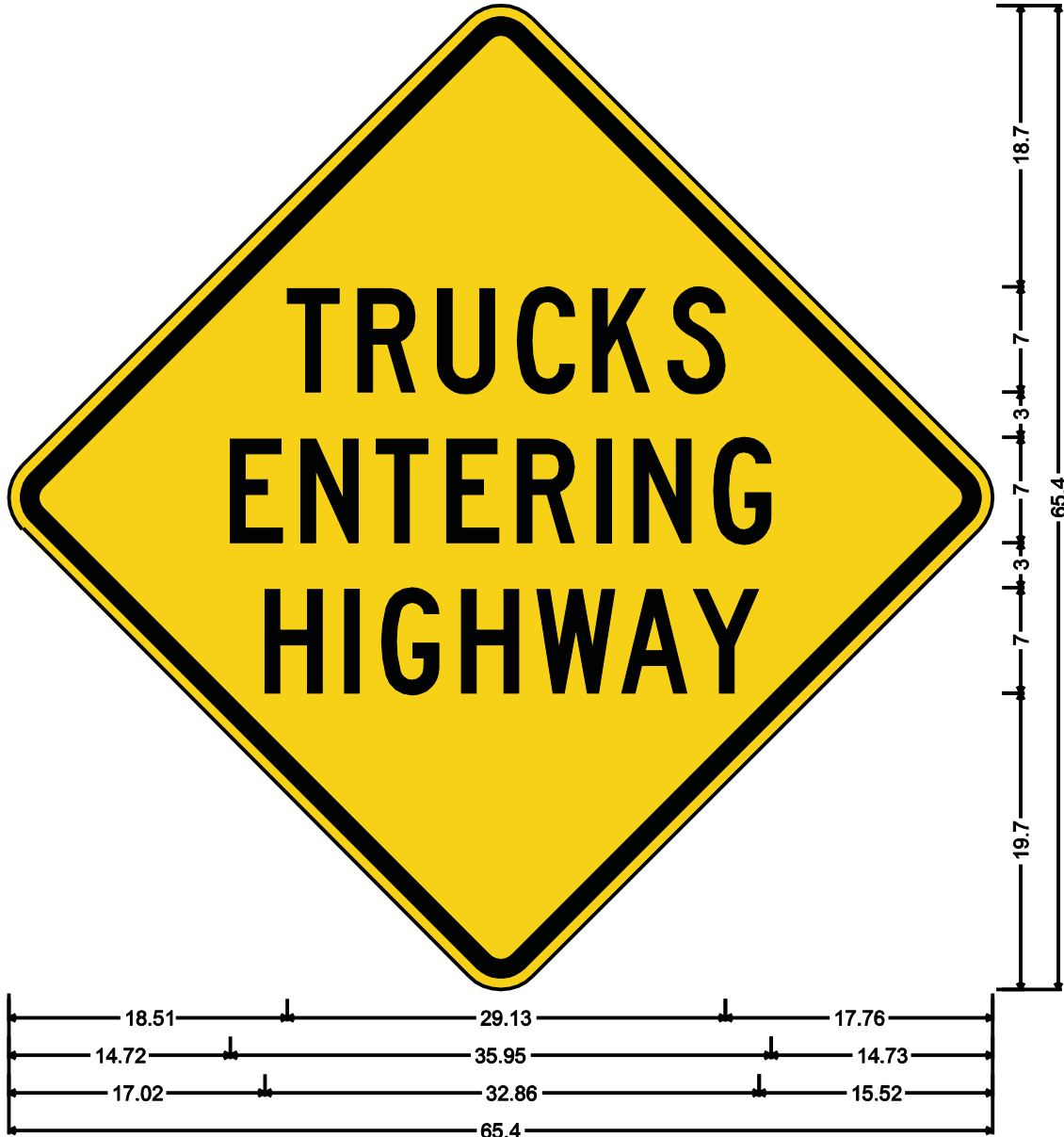
W11-13-48; 48.00" across sides 3.00" Radius, 1.25" Border, 0.75" Indent, Black on Yellow; [TRUCKS] C; [ENTERING] C; [HIGHWAY] C; Table of distances between letter and object lefts.
