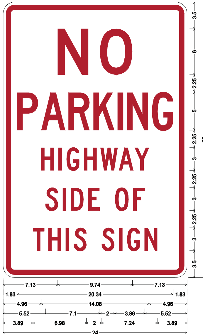
R8-1.6-24; 1.50" Radius, 0.63" Border, 0.38" Indent, Red on White; [NO] D 106% spacing; [PARKING] C 50% spacing; [HIGHWAY] C; [SIDE] C; [OF] C; [THIS] C; [SIGN] C; Table of distances between letter and object lefts.
