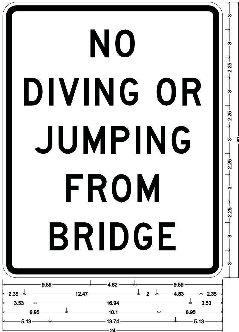
R20-1C-24; 1.50" Radius, 0.63" Border, 0.38" Indent, Black on White; [NO] D; [DIVING] D; [OR] D; [JUMPING] D; [FROM] D; [BRIDGE] D; Table of distances between letter and object lefts.
