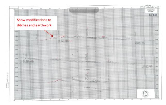
Cross section sheet depicting electronic redlining and elevations at breakpoints.
