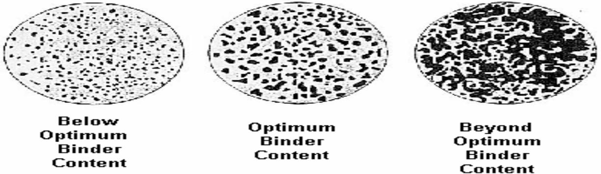
5.1.2 Perform SC-T-90 to determine the amount of binder retention at optimum asphalt binder content. This will eliminate the use of excessive binder content in the OFGC. Adjustment of optimum
