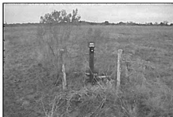
Photo 22 – MW062 two risers knocked down
