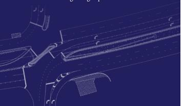
Instead, all minor road traffic makes a right turn followed by a U-turn at a designated location either signalized or unsignalized—to continue in the desired direction, as shown in Figure 1.
